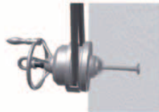
The handwheel is turned until the turning and lifting link sits tightly against the concrete.
